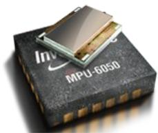
The network will be built using a number of interconnected 6DOF (3D accelerometer combined with 3D gyroscope) MPU-6050 sensors, placed at strategic locations: fingertips, back of hand, arms, chest, forehead... Data from the sensors will be gathered over serial line and software post-processed, to aggregate the raw readings of the sensors and translate them into position in time and space.
